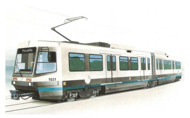
The initial system will be operated with a fleet of 26 vehicles. Up to 23 vehicles will be in service in the peak periods with the remaining 3 on standby or under maintenance, whilst 14 vehicles will be required for the offpeak service. Phase I will be operated by single vehicles but they can be coupled in tandem to provide extra capacity and, in fact, four vehicles can be controlled by a single driver in an emergency.
